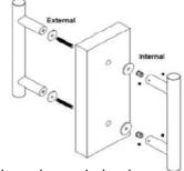
Handle(s), See opposite assemble diagram. Do not over tighten the screw threads, and check alignment once installed. Also ensure silicone is applied to the holes prior to fixing the bar handles.
